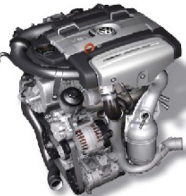
downsized engine (1.4l / 125 kW)
